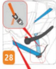
**6.4.** Insert the diagonal belt into the slot at the rear of CS128 (part no.19 page 01). (fig. 29).
